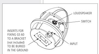
GS 60 can be placed on several surfaces, such as wood, concrete or into the ground.
